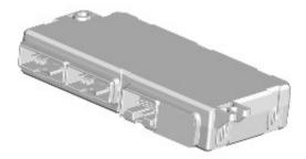
The seat modules are equipped only where seat memory is specified. On memory electric seats the seat switchpack is operated on Local Interconnect Network (LIN) bus with the seat modules.
