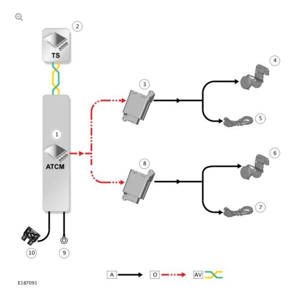
A = HARDWIRED: O = LOCAL INTERCONNECT NETWORK (LIN) BUS: AV = HIGH SPEED (HS) CONTROLLER AREA NETWORK (CAN) COMFORT SYSTEMS BUS.
