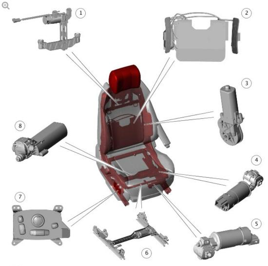
ITEM DESCRIPTION 1 Head restraint motor Seat lumbar assembly 2 3 Seat backrest recline motor Seat cushion tilt motor 4 Seat cushion extension motor 5 6 Seat forward/rearward motor 7 Seat switchpack Seat height motor 8
