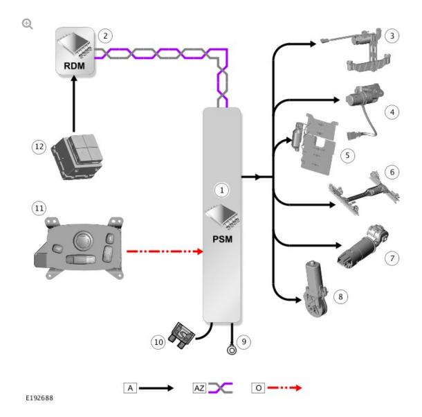
A = HARDWIRED: AZ = HIGH SPEED (HS) CONTROLLER AREA NETWORK (CAN) BODY SYSTEMS BUS: O = LOCAL INTERCONNECT NETWORK (LIN) BUS.
