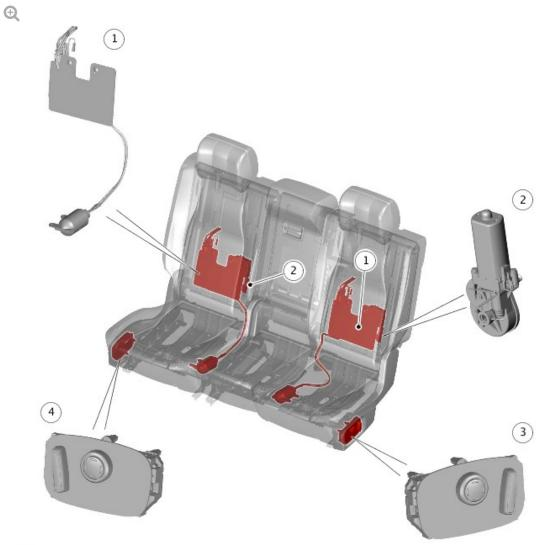
ITEMDESCRIPTION1Seat lumbar assembly (2 off)2Seat backrest recline motor (2 off)3Seat switchpack - Rear left4Seat switchpack - Rear right
