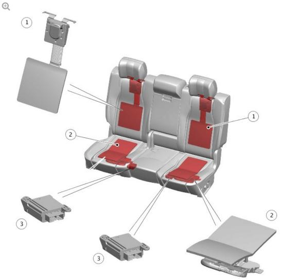
ITEMDESCRIPTION1Seat backrest climate assembly (2 off)2Seat cushion climate assembly (2 off)3Rear Seat Climate Control Module (RSCCM) (2 off)
