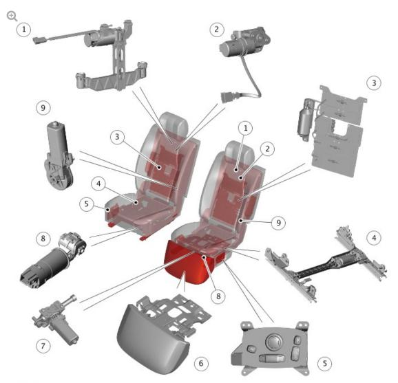
ITEM DESCRIPTION Head restraint motor (2 off) 1 2 Upper backrest adjustment motor (2 off) Lumbar massage assembly (2 off) 3 4 Seat forward/rearward motor (2 off) Seat switchpack (2 off) 5 6 Calf rest 7 Calf rest actuator 8 Seat cushion tilt motor (2 off) 9 Seat backrest recline motor (2 off)
