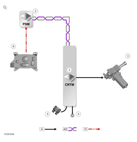
A = HARDWIRED: AZ = HIGH SPEED (HS) CONTROLLER AREA NETWORK (CAN) BODY SYSTEMS BUS: O = LOCAL INTERCONNECT NETWORK (LIN) BUS.
