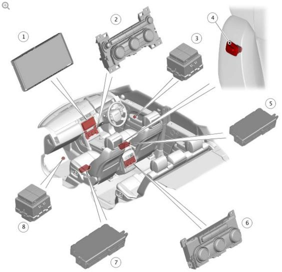
ITEM DESCRIPTION Touch Screen (TS) 1 2 Integrated Control Panel (ICP) 3 Seat memory switchpack - Driver 4 Seat away switch 5 Driver Seat Module (DSM) 6 Rear Integrated Control Panel (RICP) 7 Passenger Seat Module (PSM) 8 Seat memory switchpack - Passenger
