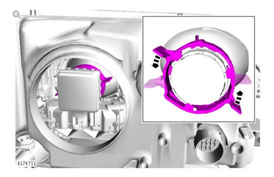
Rotate the headlamp bulb locking ring counter-clockwise.
