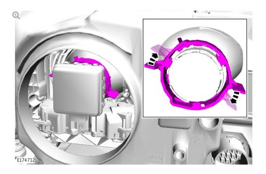
Rotate the headlamp bulb locking ring clockwise.
