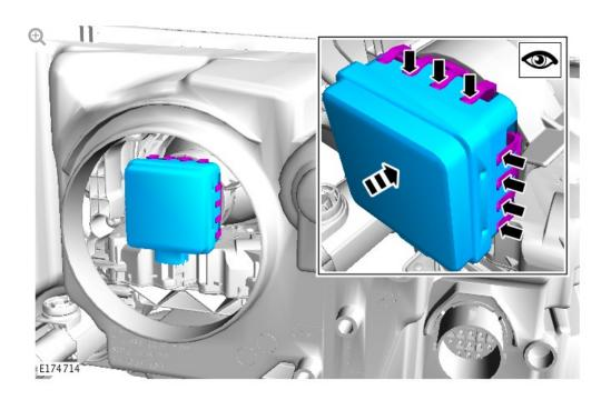
Install the headlamp bulb, make sure the spring tabs are located
