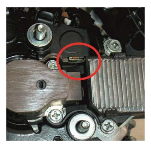
As you can see in the picture below there are two diodes that have blown apart there was a total of 5 that where in this condition.
