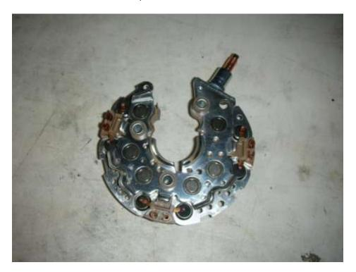
Slide the new diode pack over the three studs making sure the six copper wires come through in to the three connectors that you will now re-solder back on to the diode base plate.
