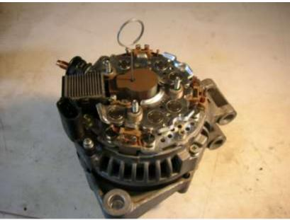
Slide the holder back on to the main shaft and secure using the two screws then once all secure pull out the pin and you should here the brushes click against the main shaft.
