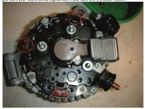
Once you have removed the solder you can now remove the diode pack from the main body of the alternator by lifting it off the three studs, you should now have this view.
