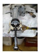
5. **Removing the old pulley**. You can now remove the pulley off quite easily. This is best done with a puller, rather than tapping the pulley off which could damage the snout bearing. Take care not to lose the clip in front of the bearing cover, and make sure you check the supercharger shaft for any marks you may have made and dress these to make sure they will not cause obstruction when you fit the new pulley.
