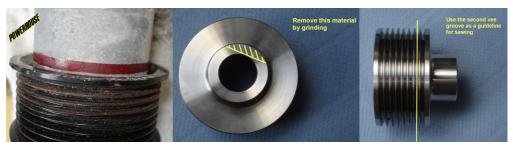
4. Grinding and cutting the old pulley. Now, using an angle grinder or other suitable tool, grind flat the front of the pulley until you just – only just – cut through the pulley to reveal the supercharger shaft beneath. You will see when you've nearly ground down to the shaft as the remaining pulley material will become thin and will start to discolour due to heat. Do this all the way back to the where the pulley diameter increases.
